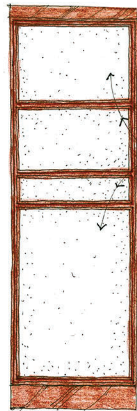
MUSIC ROOM - SEPARATE PANELS REAR VIEW OF SLIDING PANEL CREATED BY RECESS
